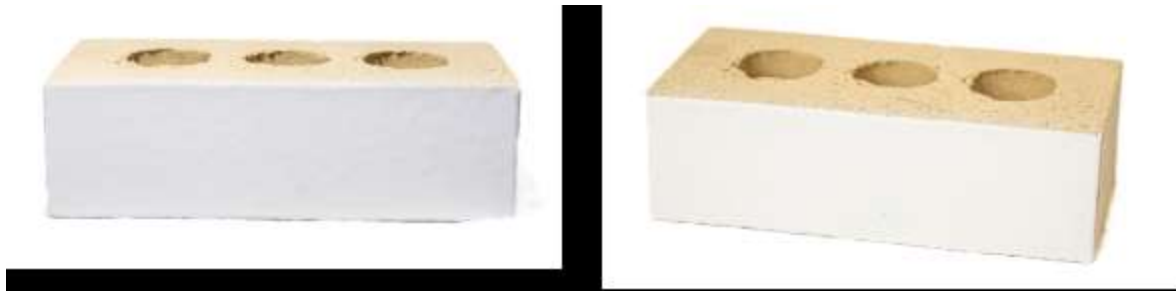
Figure 1 - Example of White Glaze on Brick Face
