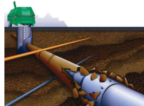
PNEUMATIC PIPE BURSTING
