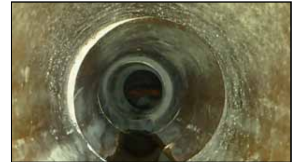
HD CRAWLER SYSTEM CRISPLY STARES DOWN THE BARREL OF THE SMALL DIAMETER PIPE TO THE UPCOMING MANHOLE.
