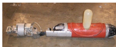
Typical bladder used for resin injection. The heat shield is indicated in red.
