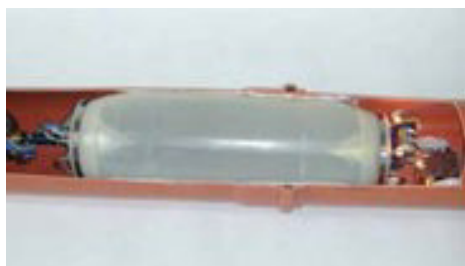
Translucent Bladder for UV Curing of Sectional Liner
