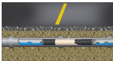
Sectional liner being positioned in pipeline
