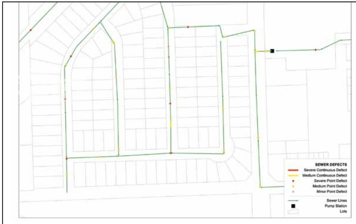
Figure 1: Structural Pipe Ratings (Green=Good, Yellow=Re-inspect, Orange=Repair if budget allows, Red=Emergency Repair)
